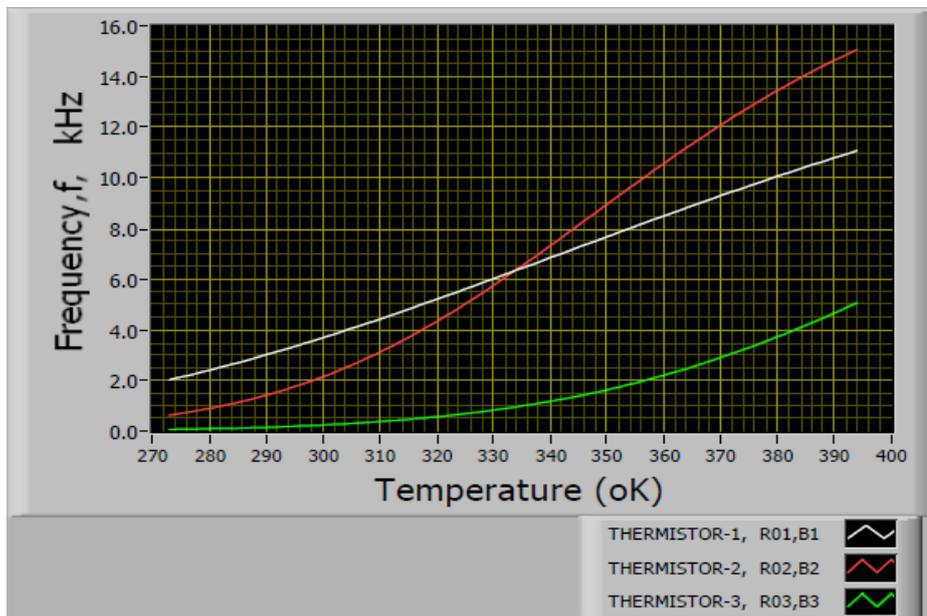
Fig.5. Simulated characteristic of thermistor ( $R_T=1000\Omega$ ,  $C_T=120nF$ )
