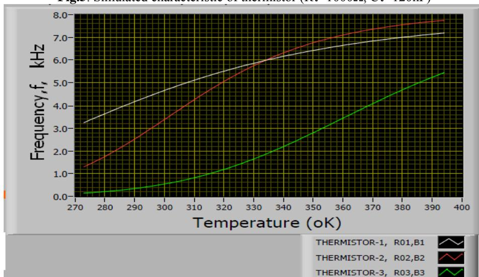
Fig.6. Simulated characteristic of thermistor ( $R_T=6000\Omega$ ,  $C_T=50nF$ )
